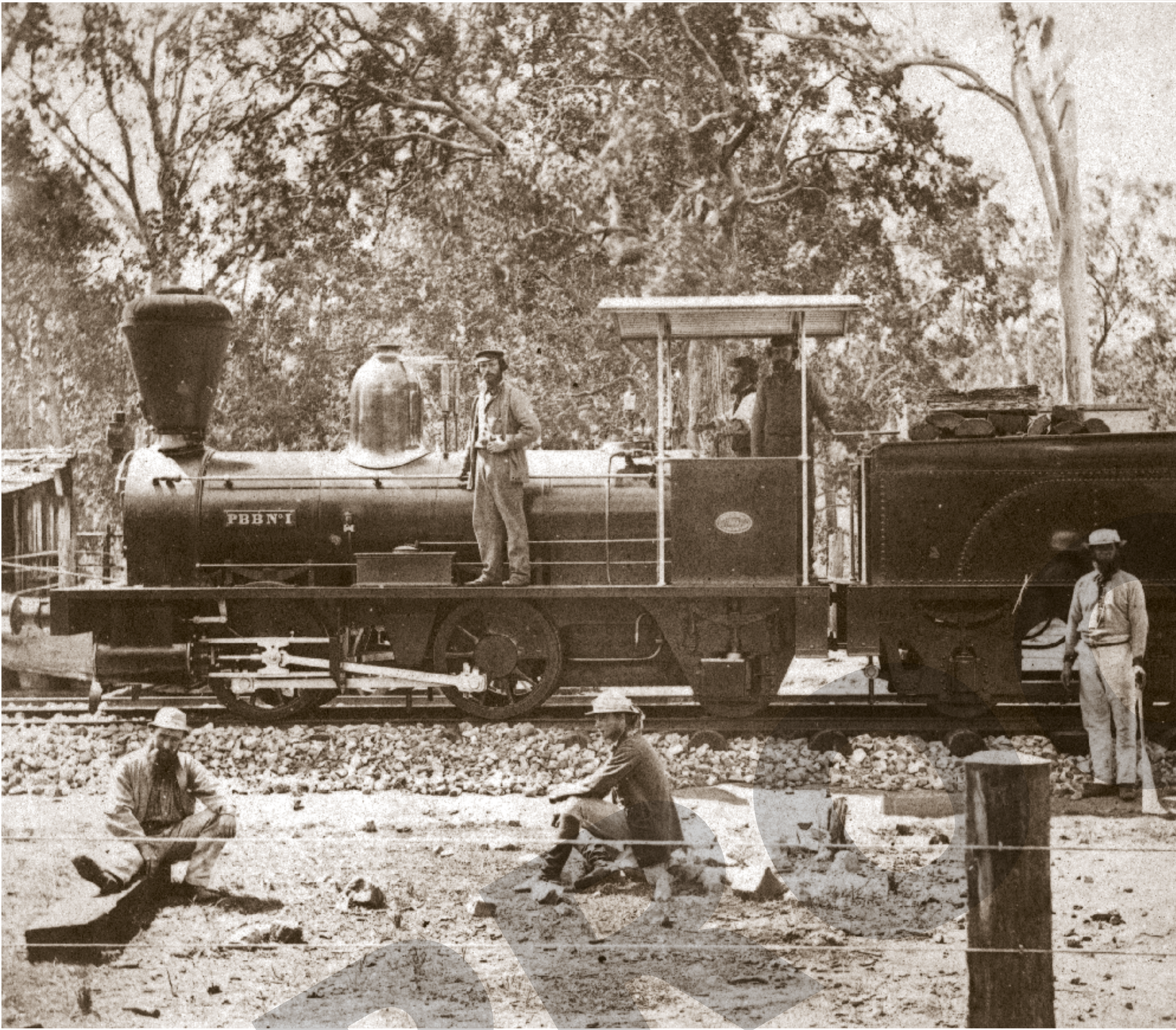
One of the original wood burning A10's No 4, or PBB No 1, the contractors locomotive.
