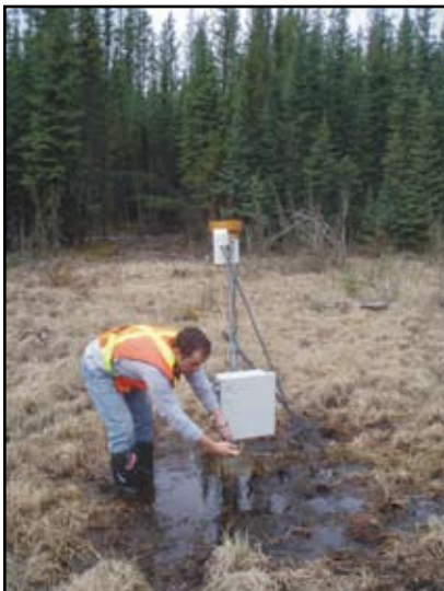
Installing a climatic station on MEG's lease to collect rainfall and air temperature data during 2007.
