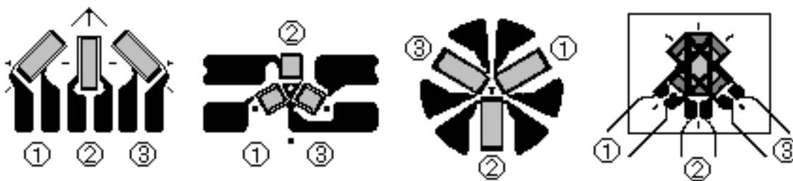
Counterclockwise numbering of gage grids in Micro-Measurements general-purpose strain gage rosettes.
