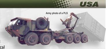
truck with self load/unload capability. The PLS carry payload on flat rack cargo bed, trailer, or International Standards Organization (ISO) containers. The HEMTT is a 10-ton, 8 wheel (8x8) truck that comes in several configurations: The Tanker to refuel tactical vehicles and helicopters, Tractor to tow the Patriot missile system and Multi-Launch Rocket System (MLRS), Wrecker to recover vehicles, and Cargo truck with a materiel handling crane. The HEMTT entered service in 1982.
