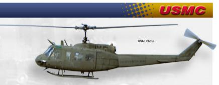
The upgraded helicopters will have increased maneuverability, speed, and payload capability. The upgrade scope includes a new four-bladed rotor system, new transmissions, a new four-bladed tail rotor and drive system, and upgraded landing gear.
