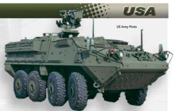
There are two basic versions, which include the Infantry Carrier Vehicle (ICV) and the Mobile Gun System (MGS). There are eight different configurations, which include the Reconnaissance Vehicle (RV); Anti-Tank Guided Missile (ATGM); Nuclear, Biological, Chemical, and Radiological Vehicle (NBCRV); Medical Evacuation Vehicle (MEV) Commander's Vehicle (CV); Fire Support Vehicle (FSV); Mortar Carrier (MC); and Engineer Squad Vehicle (ESV).
