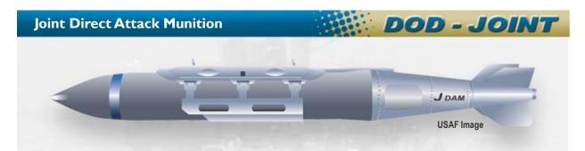
The Joint Direct Attack Munition (JDAM) is a joint Air Force and Navy program led by the Air Force. The JDAM improves the existing inventory of general purpose gravity bombs by integrating a Global Positioning System (GPS)/inertial navigation guidance capability that improves accuracy and adverse weather capability.
