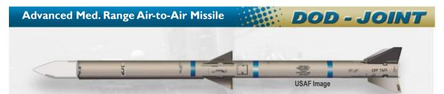
The Advanced Medium Range Air-to-Air Missile (AMRAAM) is an all-weather, allenvironment radar guided missile developed to improve capabilities against very lowaltitude and high-altitude, high-speed targets in an electronic countermeasures environment. The AMRAAM is a joint Navy/Air Force program led by the Air Force.
