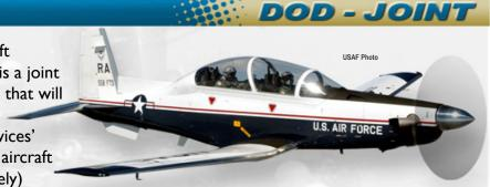
and associated Ground Based Training Systems. The T-6 Texan II is a tandem seat, turboprop aircraft derivative of the Pilatus PC-9 powered by a single Pratt & Whitney PT6A-68 engine.
