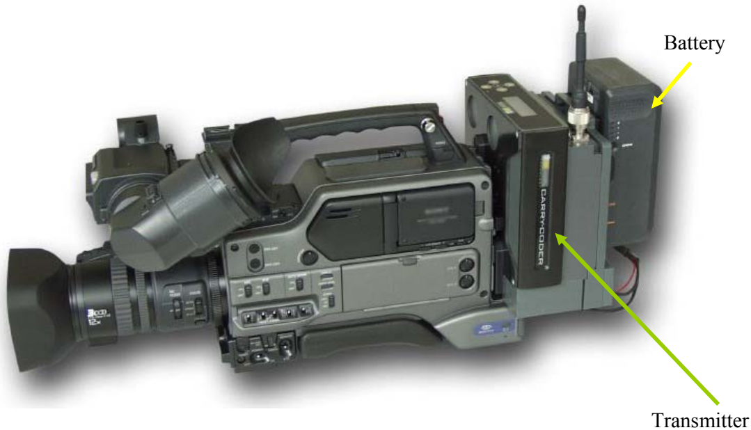
Fig. 4 ENG Camera with the TX attached
