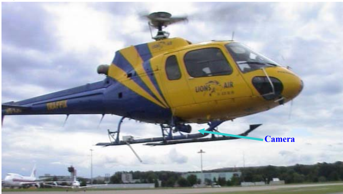
Fig. 6, Wireless camera mounted at a helicopter
