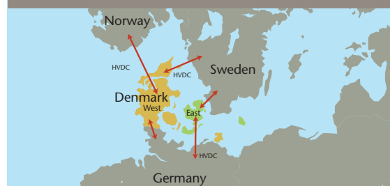
Figure 9.1 Denmark is interconnected with Norway, Sweden and Germany. An HVDC link between west and east is under construction.
