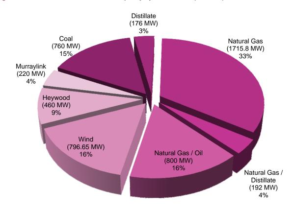
Figure 4-1 - South Australian Installed Capacity by Fuel Source (2009-10<sup>6</sup>)
