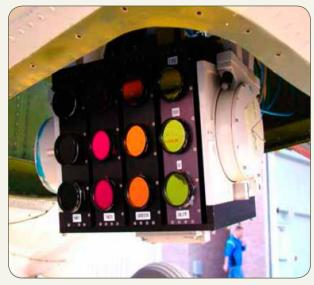
Airborne Remote Optical Spotlight System Multispectral Polarimeter (AROSS-MSP)
