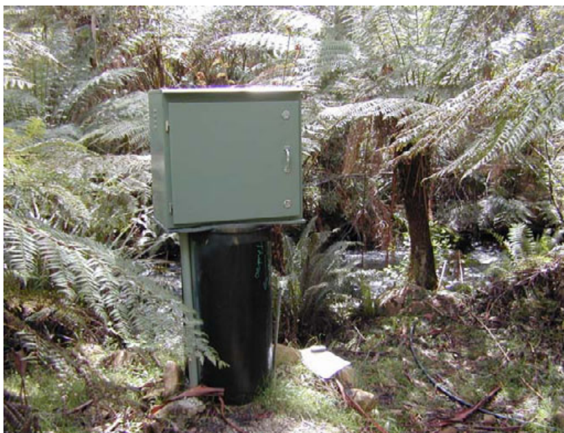
Figure 2.11. The gauging station on the Cement Creek.
