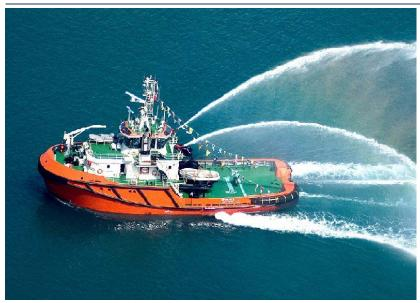
The new tugboat Spinola, christened by was Catherine Gonzi last week. The new 80 tonnes Bollard harbour escort/terminal tug is the latest addition to Tug Malta's present fleet of six modern tugs. It was ordered from the Spanish Shipyard Armon S.A. and was primarily designed to operate in the Maltese harbours and their approaches. The tug is fully equipped with Fire-Fighting
