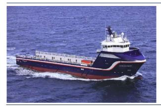
STX Europe delivered its newbuilding No. 726 **Highland Prince** from the Søviknes yard to Gulf Offshore N.S. The vessel is designed as a platform supply vessel for world wide operations and for transport of general cargo for the offshore industry. (Source & Photo STX Europe)
