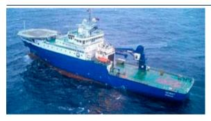
Norway-based DOF Subsea has won contracts worth US\$22 million for its multi-role support vessel, 'Geobay'. The vessel will be deployed for construction work on Australia's northwest shelf until mid December. 'Geobay' is a DP 2 vessel with a length of 85.45 metres, a beam of 15.6 metres and a draught of 6.9 metres. The 3,502GT vessel can achieve a maximum speed of twelve
