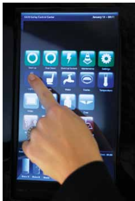
Each seat in the G650 comes with its own iPod Touch passenger control unit. Crewmembers will select all the galley functions via controls presented on a 10-inch touch screen (above).
