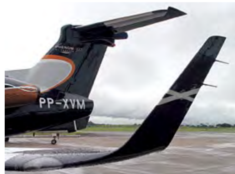
The swept wing of the Phenom 300 is one indication that the light jet is a clean-sheet design, rather than merely a stretched version of the Phenom 100.
