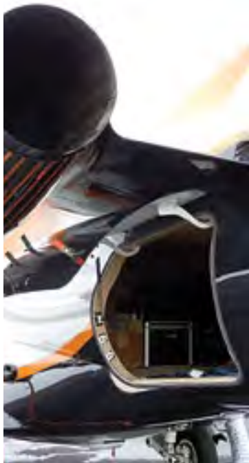
The 66-cu-ft rear baggage compartment offers plenty of room for the passengers' bags and other gear.
