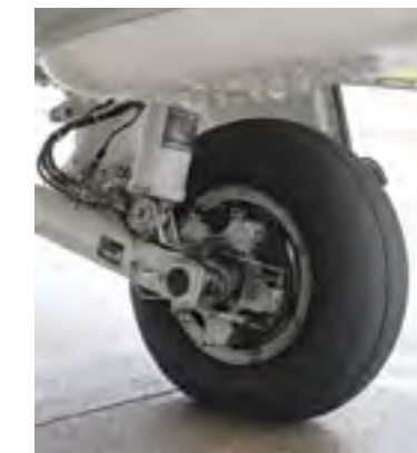
Like its smaller sibling, the Phenom 300 has trailing-link main gear with brake-by-wire and an anti-skid system that should help even new pilots deliver smooth landings.
