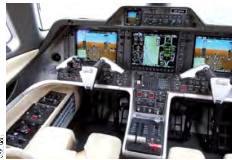
The Phenom 300's Prodigy flight deck is based on Garmin's all-glass, fully integrated G1000.
