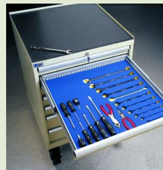
The two liners protect tools and make missing ones easy to notice.
