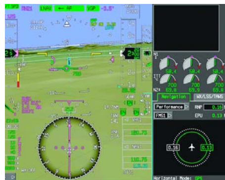
Honeywell is continuing development of its synthetic-vision display for Dassault's EASy II cockpit.
