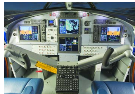
Viking's Twin Otter revival of the de Havilland Canada workhorse features a Honeywell Primus Apex in the front office.
