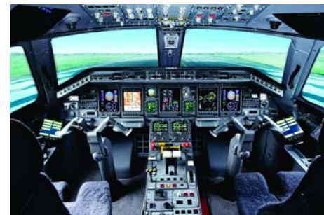
Honeywell's Primus Elite can be retrofit into legacy aircraft with CRT screens, and it will also serve as the avionics for the in-development Legacy 650.
