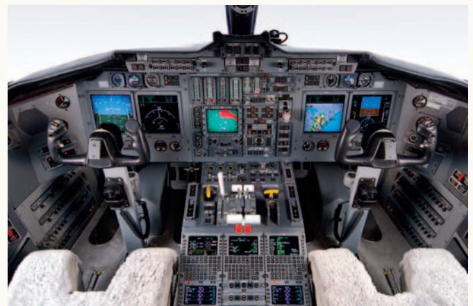
This Challenger 601-3A owned by Universal Avionics is undergoing final flight testing for the Vision 1 SVS portion of the airplane's EFI-890R cockpit.
