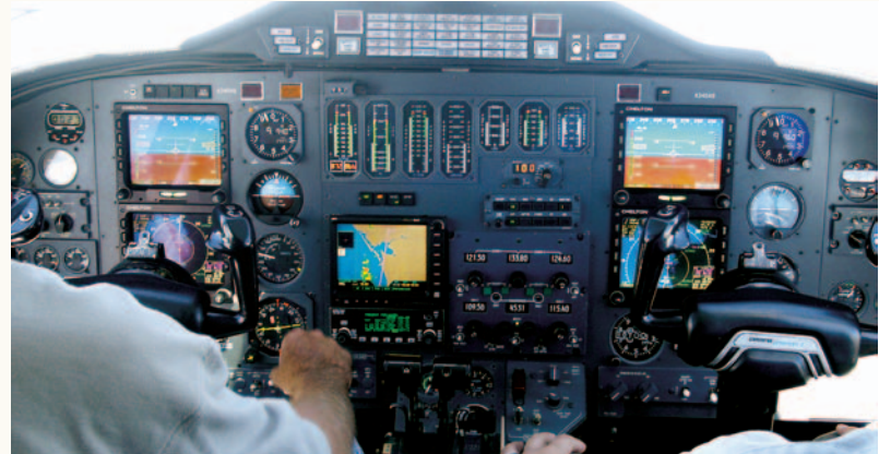
The first SVS certified for civil airplanes, Chelton's FlightLogic EFIS has found a niche in business aviation, recently with a STC for installation in the Cessna Citation 501.
