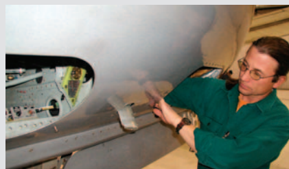
NASA researcher Taumi Daniels checks the weather sensor installation in a Saab 340, left. Mesaba's fleet has been fitted with the devices.
