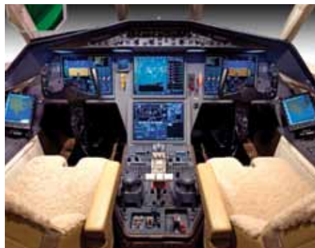
Dassault's EASy cockpit avionics are built on the Honeywell Primus platform.
