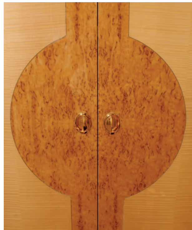
Exotic woods are commonplace in the business jet cabin, such as the inlay work on these cabinet doors in a 767-300 recently delivered by Gore Design Completions. Veneer on the main door is quarter-cut sycamore and the oval inlay is karelian birch burl.
