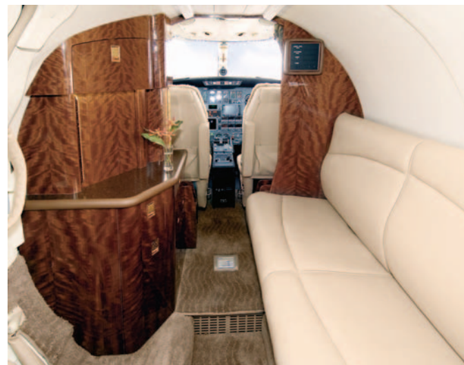
Duncan Aviation's interior designers have become adept at creating galley and refreshment centers that make the most of limited interior space, such as the galley placement just forward of the cabin door in this Citation Encore.
