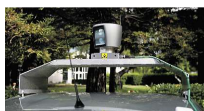
The laser on the roof of one of the self-driving vehicles Google is developing.
