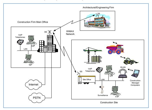
The fast deployability of WiMAX networks is also important in this scenario, since it allows for quick provision of communications to the construction site, including voice (telephony) and data (emails, engineering drawings, and Internet access). Surveillance video can also be carried over the network, to support monitoring of the site or areas of the site that are otherwise difficult to access. A local Hotspot can also be set up at the
