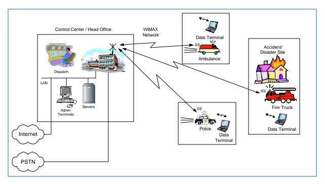
In addition to providing two-way voice communications between the dispatch center and on-site emergency response teams, the network relays video images and data from the site of the accident or disaster to the control center. This data can be relayed to expert teams of medical or emergency staff, who can analyze the situation in real-time, as if they were on site. WiMAX QoS allows the network to handle these diverse types of traffic.
