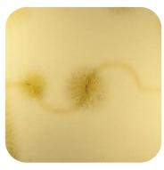
Appearance of the patch with defect visible as a snowflake pattern
