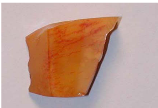
Figure 5.9 Baltic amber aged on an open dish at 100 °C for 35 days has a high concentration of red veins, particularly around edges. Sample is approximately 30 x 30mm.
