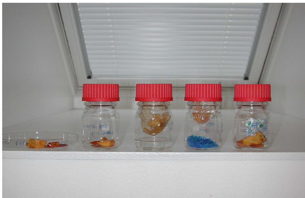
Figure 4.3 Experimental storage environments used to thermally age amber. From left to right: open ageing, closed, high RH, low RH, oxygen-free
