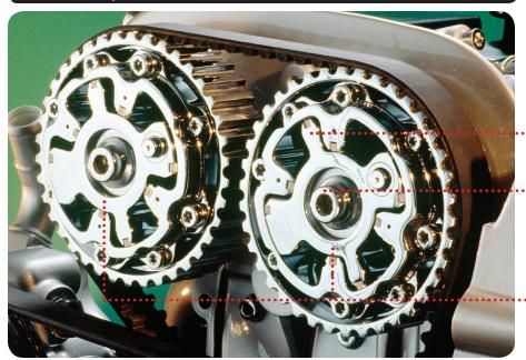
Electronic solenoid valves direct high-pressure engine oil to control vanes in each of the camshaft sprocket housings.
