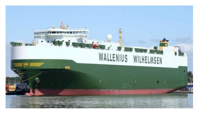
The LCTC (Large Car Truck Carrier) m/v ANIARA has a capacity of 8,000 cars or a combination of 3,484 cars and 466 buses. With her 231.6 metres and 71,673 gross tonnage she is the world's largest car carrier. The vessel is built to the highest class of Lloyd's Reg-
