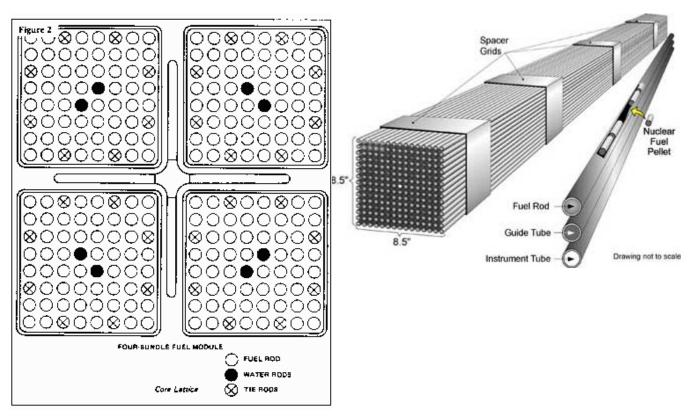
A diagram of a typical nuclear reactor fuel assembly is shown in Figure 2 (from Knief, 1990).
