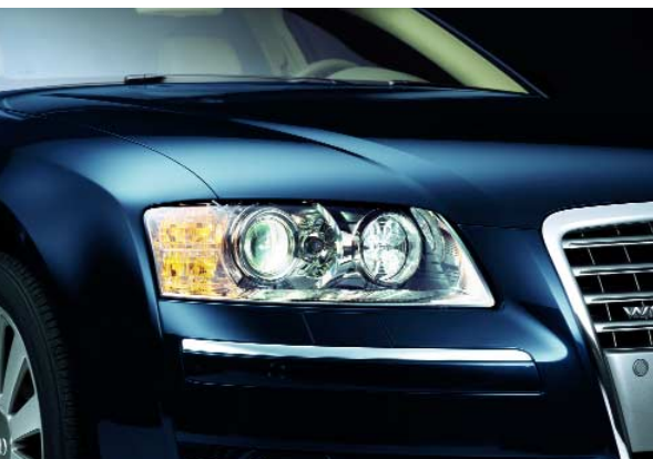
Headlights in the Audi A8 L 6.0 quattro with LED daytime driving lights
