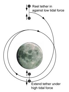
**Figure 10.** Schematic of tether reeling maneuver to reduce orbital eccentricity.
