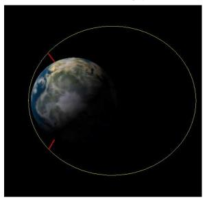
**Figure 6.** The HEFT Boost Facility's initial orbit. The red lines indicate the bounds of the perigee portion of the orbit where electrodynamic thrusting is effective.
