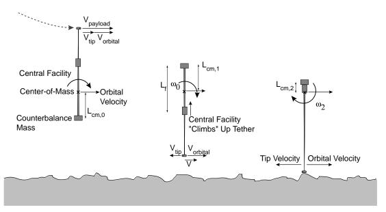
Figure 8. Method for a lunar tether to capture a payload from a minimal-energy LTO and deposit it on the Moon with zero velocity relative to the surface.
