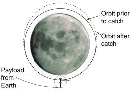
Figure 9. Lunavator™ orbits before and after payload capture.
