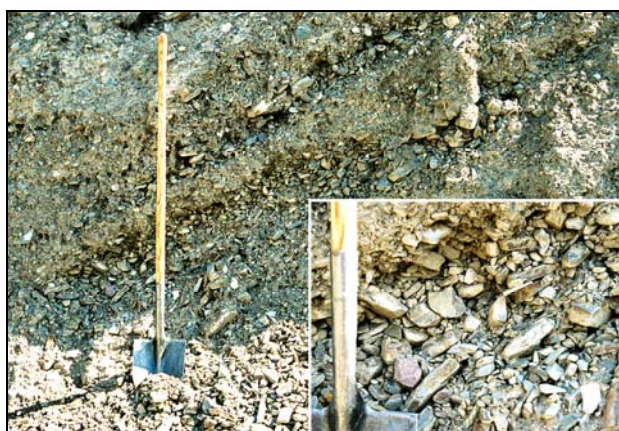
Figure 42—Gravels in expansion bar show crude foreset beds dipping 29°. Note open-work cobble-pebble gravel.
