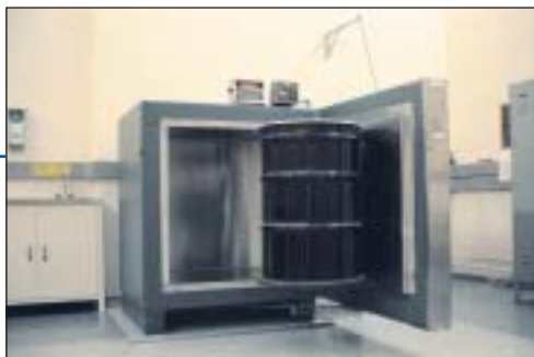
SCK•CEN uses a Q 2 test system for low-level waste in order to measure the radioactivity.
