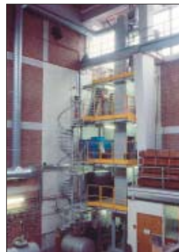
In order to eliminate tritium from liquid effluents of a reprocessing plant, SCK•CEN developed the ELEX process.
