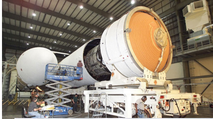
First and Second Stage Mate in the HIF
