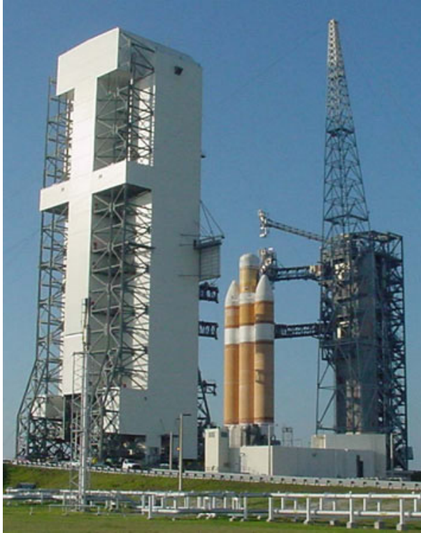
Figure 8. Tanking Test 1 – Simultaneous CBC Loading
