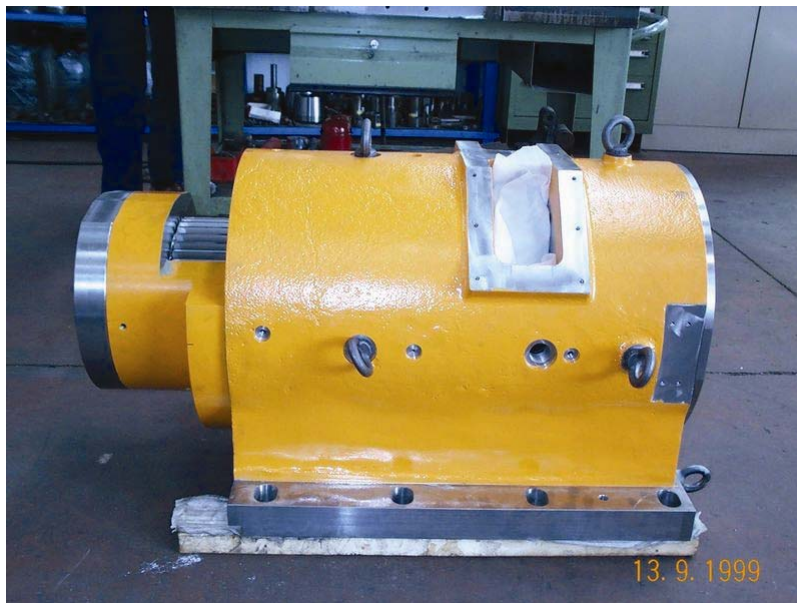
Figure 7-36. Photo of LBT drive motor housing.
