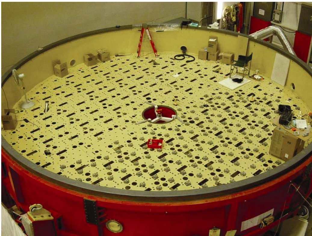
Figure 7-9. View of top plate of LBT mirror cell. GMT top plate will be similar.
