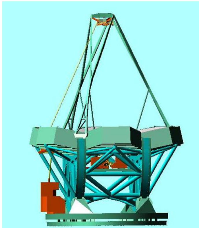
Figure 9-36. View showing the laser optics. Six sodium laser beacons are housed in the room on the az-platform (lower left). The beams are directed to a projector above the secondary via two flat mirrors on the elevation axis. The platform-mounted AO instruments are visible directly below the primary mirror assembly.
