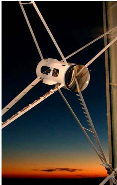
Figure 9-13. MMT deformable Cassegrain secondary, mounted in the telescope at sunset.
