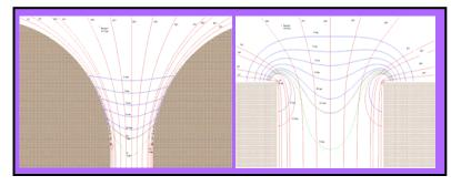
These images are from a Simion model and show the magnitude of the E field off rounded and square electrodes. The red lines show potentials, while the blue show electric field.
