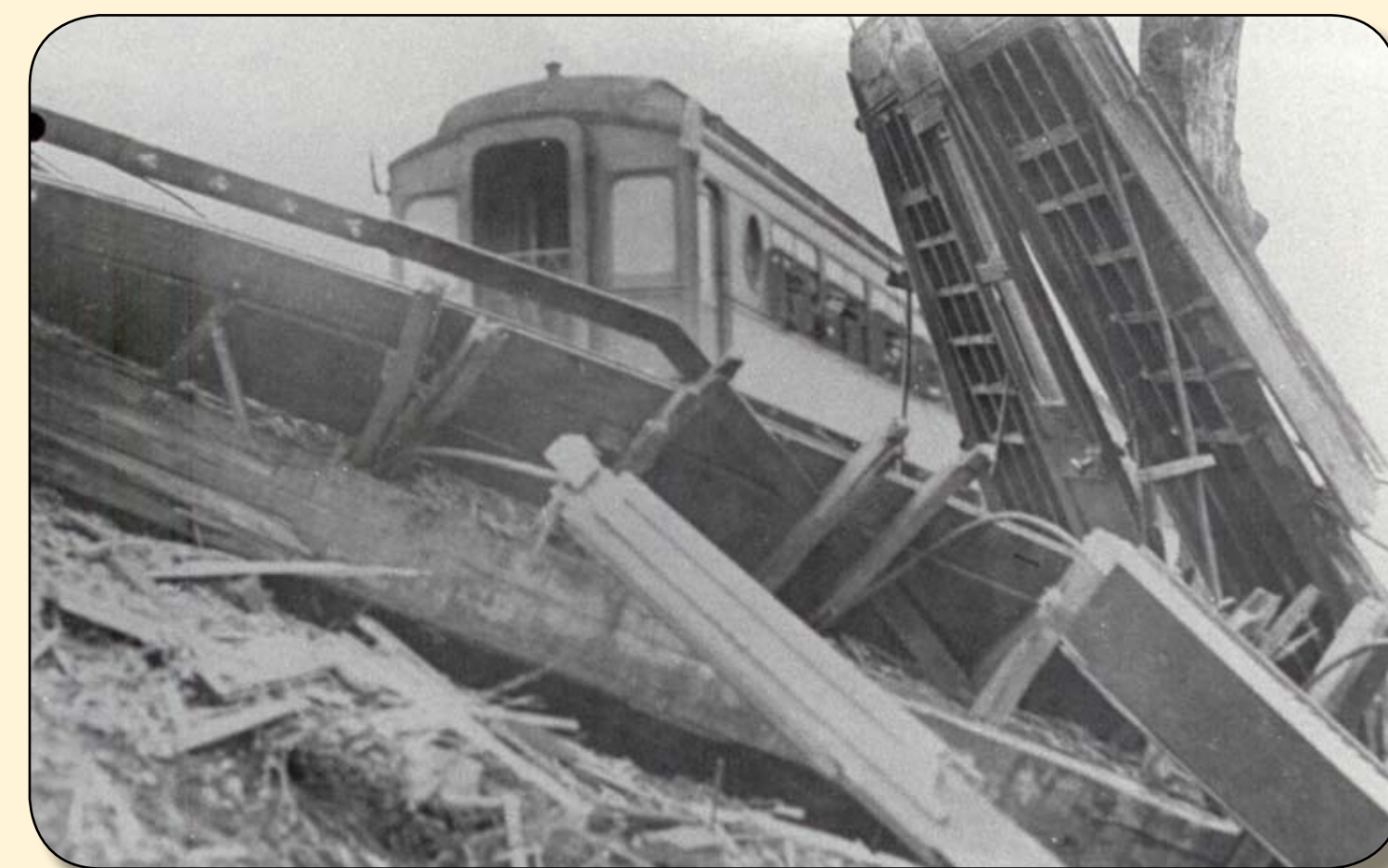
The splintered wooden framework of a passenger car.
