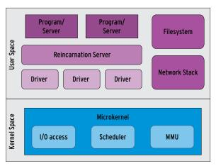
Figure 1: The Minix microkernel encapsulates many subsystems in user space, including drivers, the filesystem, and the network stack. The kernel just runs critical functions, such as underlying I/O, schedulers, and memory management.
