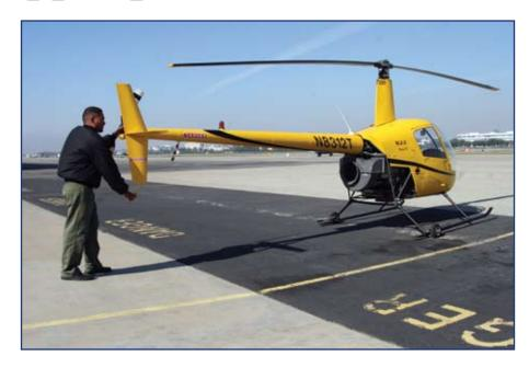
**Easy Ground Handling.** Light empty weight allows easy manual ground handling by one person. A convenient tow cart adaptor is also provided for use with the Robinson Electric Tow Cart.
