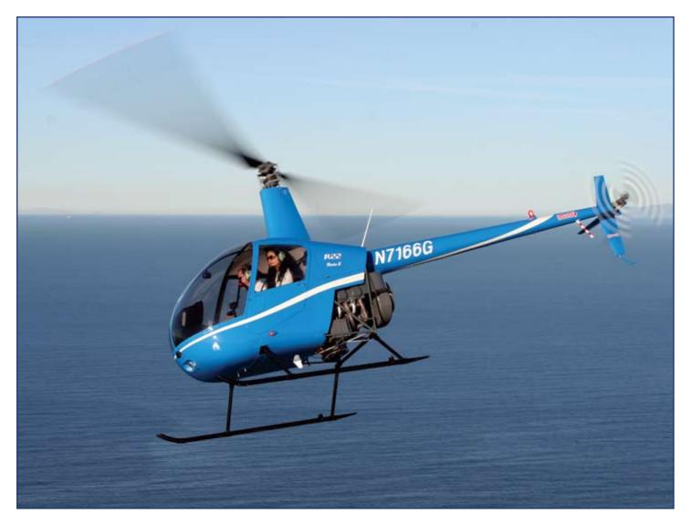
**Reliable Engine.** The dependable Lycoming O-360 engine is derated to 131 horsepower for take-off and 124 for cruise, giving the engine long life and unmatched reliability.
