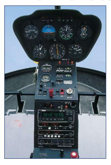
Advanced Warning Devices. The instrument panel includes low fuel warning light, main gearbox temperature and chip lights, tail gearbox chip light, low oil pressure light, engine fire light, low voltage alternator light, low RPM warning light and horn, plus rotor brake and starter engaged warning lights.
