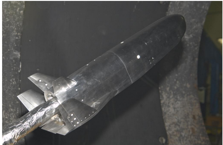
One of six hypersonic vehicle configurations recently wind tunnel tested as part of the High Alpha Reusable Launch Vehicle (RLV) Aerodynamic Configuration Development program.
