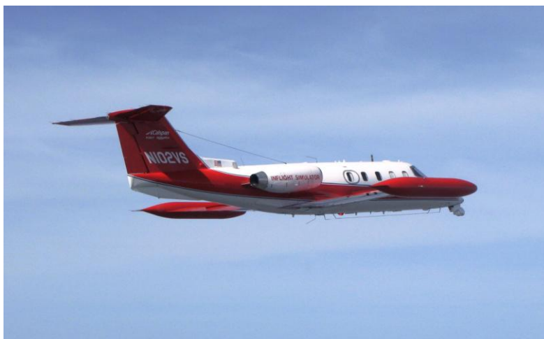
The Sense and Avoid (SAA) test platform flies above the Niagara International Airport during the recent Multiple Intruder Autonomous Avoidance flight test. The test vehicle is a Calspan Learjet equipped with the electro-optical cameras, AI-130 radar, and airspace deconfliction technologies that make up the SAA system (Calspan photo).
