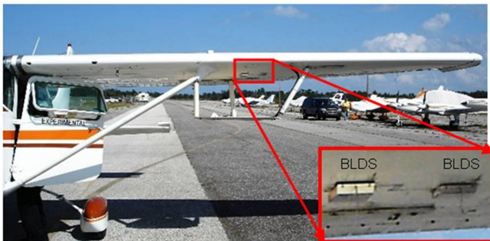
The Boundary Layer Data System, attached to the wing of a test aircraft in preparation for the latest round of flight tests.
