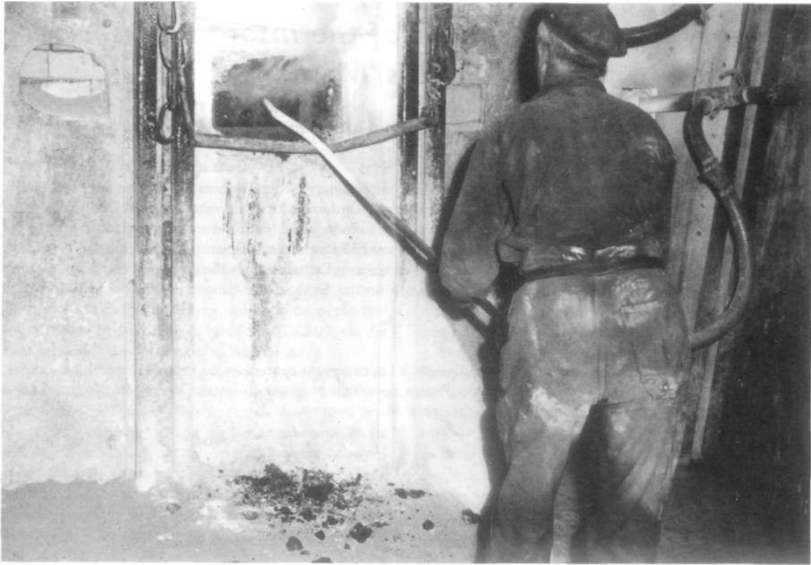
Antimony process worker in the 1960s showing the oxide fume from a furnace. Conditions were later markedly improved.
