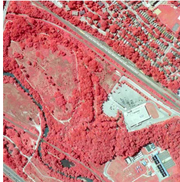
Geospatial Information: 2006 stereo colour infrared photography was interpreted to identify natural heritage community boundaries, to ascertain changes between current conditions and the previously mapped database, and to provide direction for field investigations.
