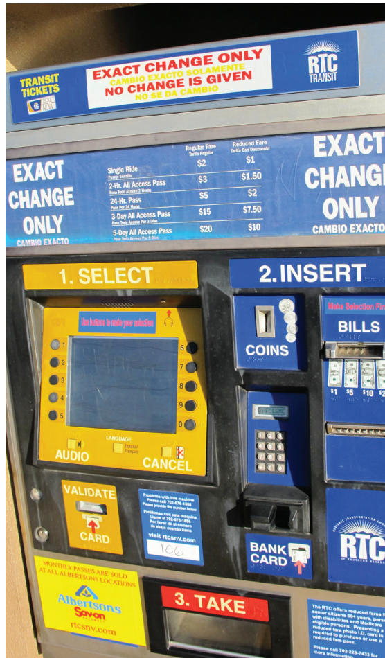
Off-vehicle fare collection machine in Las Vegas, Nevada. Photo: Annie Weinstock, ITDP
