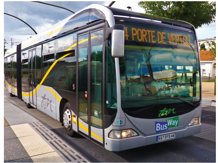
Including more than two doors, like this vehicle in Nantes, France, allows for faster boarding and alighting (above). Photo: Luc Nadal, ITDP
