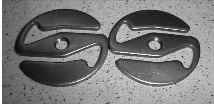
Figure 5-7 Two S-clutches from a Homelite Versatool string trimmer. The outer diameter of the clutches is 2.41 inches.
