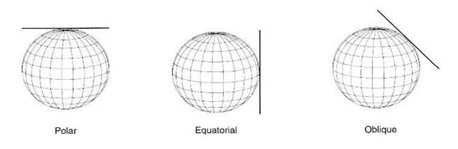
Polar projections have a dartboard arrangement of concentric lines of latitude and radiating meridians.
