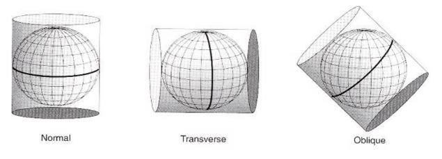
The **Mercator** projection is probably the best known projection of all. It produces a graticule with 90 degree angles. The meridians are equally spaced, whilst the spacing of the parallels (i.e. lines of latitude) increases towards the poles. The Mercator projection preserves direction, but results in massive distortions of some of the other properties (especially area in the polar regions).
