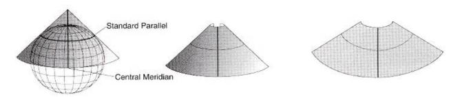
The simplest conic projection is tangential to the globe along a line of latitude (known as the **standard parallel**). The lines of latitude and longitude are projected onto the cone, and the cone is then metaphorically cut along any meridian. The opposite meridian becomes the **central meridian** in the map. The other meridians converge towards a point, and the lines of latitude appear as concentric circular arcs.
