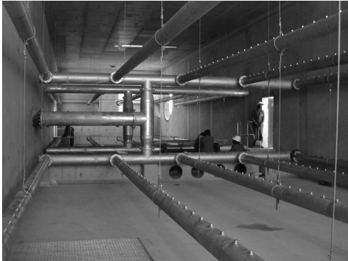
Figure 4. Internals of typical spray chamber (Wilson, 2003)
