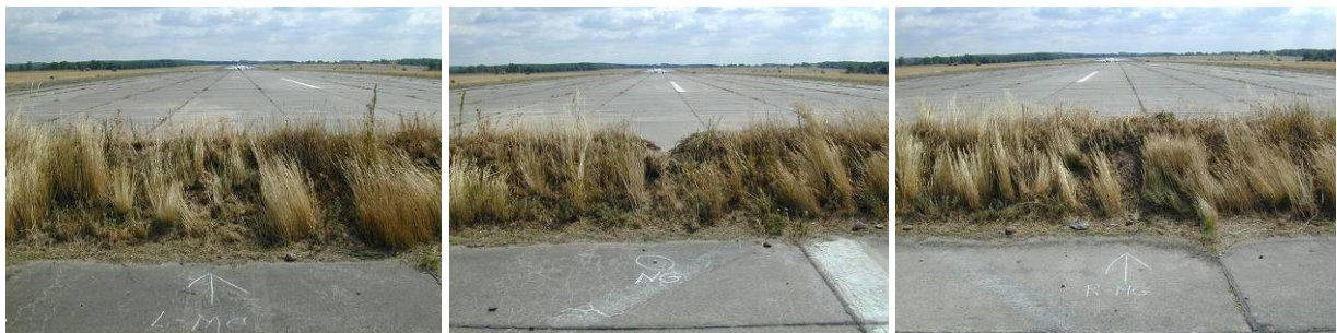
The west side of the approximately 70 cm high earth wall with impact marks: left, that of the left main landing gear; centre, that of the nose gear; right, that of the right main landing gear.
