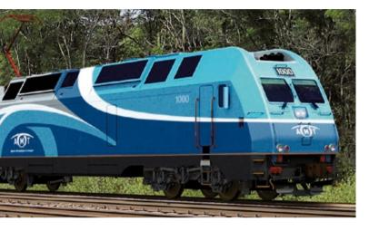
The BOMBARDIER\* MITRAC\* Hybrid enables vehicles to operate with comparable efficiency on electrified tracks as well as on non-electrified tracks. This is made possible with a common propulsion chain that is capable of utilizing both electric and diesel power sources. Customer benefits include minimal use of fossil fuels, low emissions and economic and flexible allocation of the fleet.
