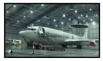
➤ Main Chamber (MC): This chamber is the largest of the testing chambers at the McKinley Climatic Laboratory and is the largest environmental chamber in the world. It is approximately 252 feet wide and 260 feet deep and 70 feet high. The immense size allows testing of very large items and complete systems. The MC has accommodated the B-2 bomber and the C-5 Galaxy, the largest aircraft in the U.S. inventory.
