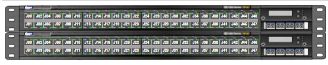
Figure 7-6 Two 1000BASE-T TOR switches
