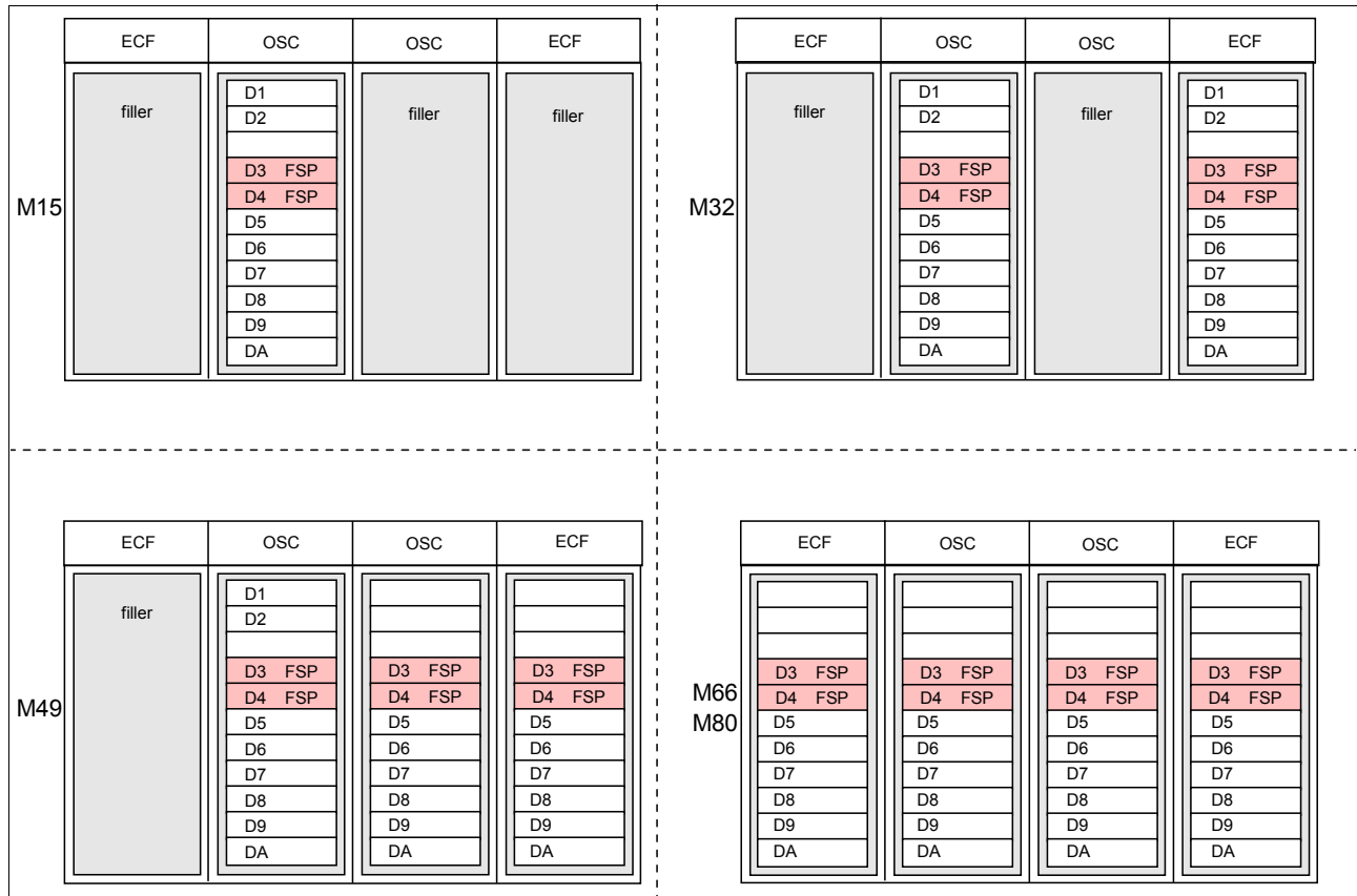
Figure 4-6 Fanout plugging rules
