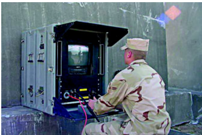
A1C Jamie Erickson operates the All-purpose Remote Transport System (ARTS) from a safe area using the Operator Control Unit. (Photos by MSgt Robert C. Hodges)
