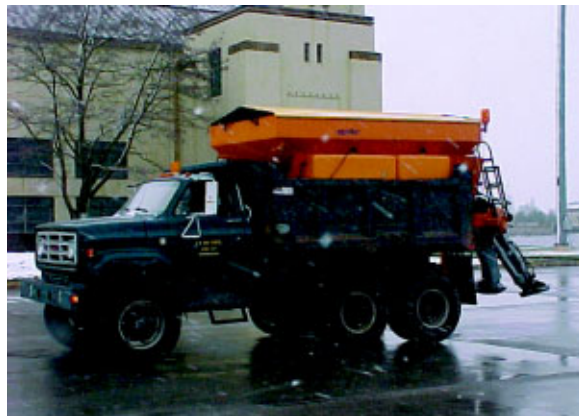
The spreader (left), grip tester (bottom right) and sprayer (bottom left) are the three components of SNIC, the newly adopted snow and ice control integrated system, which uses computers and precision sprayers to control the rate of chemicals being applied. (Photos by Jerry Adamietz)
