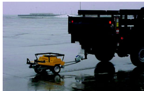
The spreader (left), grip tester (bottom right) and sprayer (bottom left) are the three components of SNIC, the newly adopted snow and ice control integrated system, which uses computers and precision sprayers to control the rate of chemicals being applied. (Photos by Jerry Adamietz)
