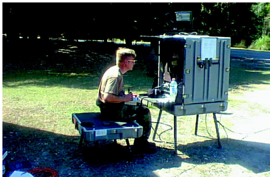
SrA Lenny Eckstein directs the ARTS' movements using joysticks and a monitor at the control station.
