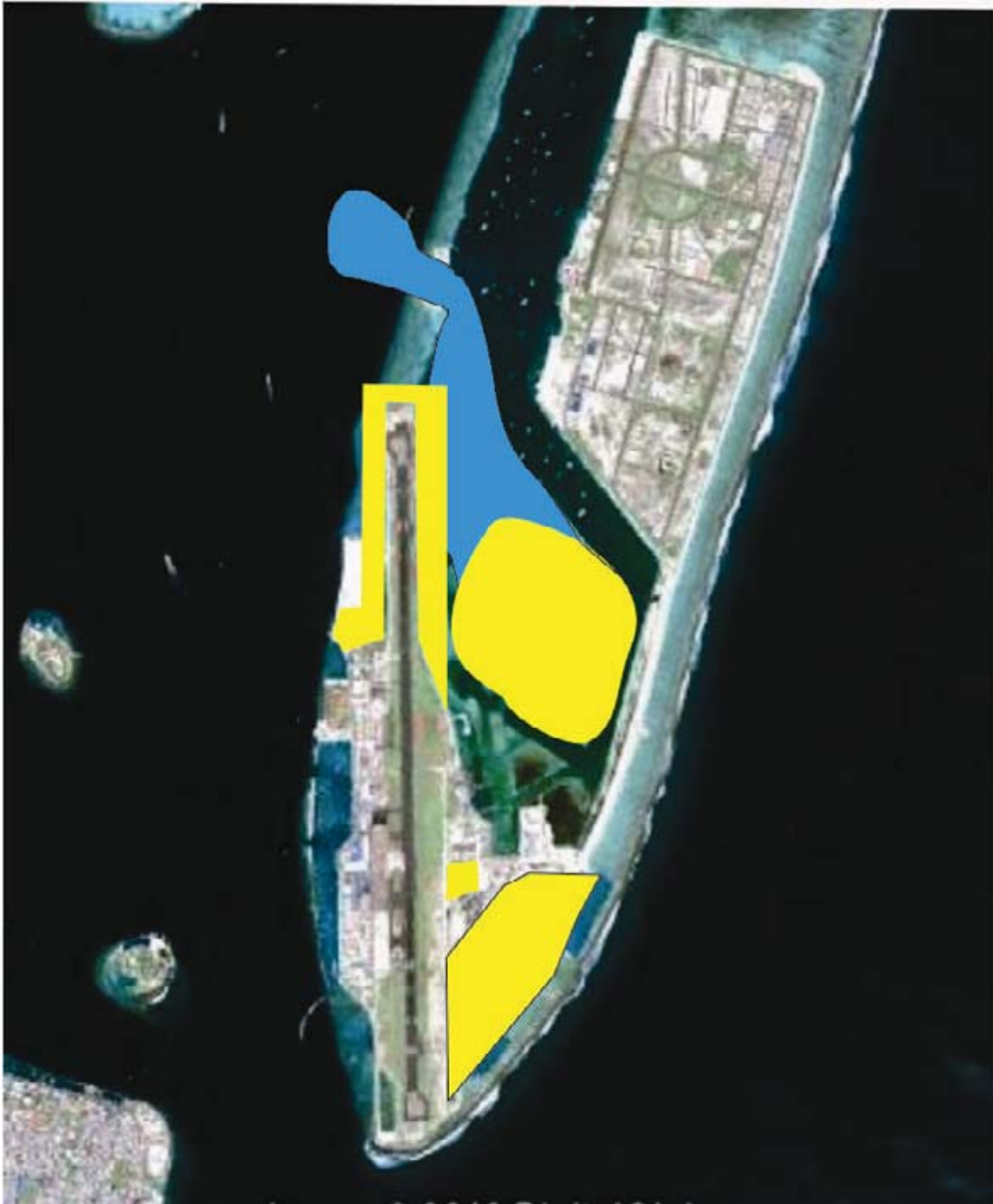
Figure 6.3: Possible area of direct influence (yellow) and less direct influence (blue shades) of suspended solids released from the proposed borrow area and reclamation area under worst case conditions
