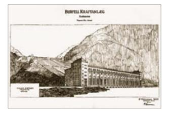
to produce electricity which would mainly be utilized for fertilizer production. He envisaged five stations on Thjórsá from the Urridafoss falls and upriver beyond Búrfell, as well as a station at Hrauneyjafoss on the River Tungnaá. Búrfell would have been by far the largest station. The plan was to dam Thjórsá at Klofaey and divert the water through an open channel into Bjarnarlón and to an intake dam at Sámsstadaklif.
